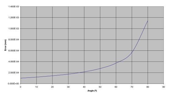
A sine bar is only used for angles less than 45°. As can be seen from the graph the error increases rapidly after 45°.
