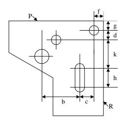
f and g are measured using the height gauge from sides R and P respectively to the top of the plug gauge  $(d_3)$ .
