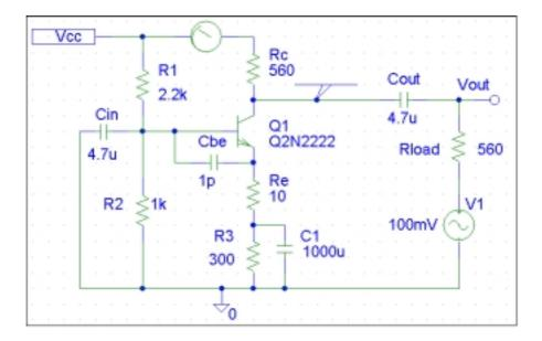
AC analysis was run and Zo was calculated as follows:  $\frac{V_{out}}{R_{load}} = Z_o$  .
