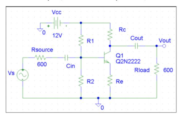
Since output impedance =  $\frac{1}{h_{cc}} \parallel R_c$  and  $\frac{1}{h_{cc}}$  is very large it can be assumed that
